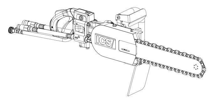
880/890 FLUSH Series Hydraulic Concrete Saw
